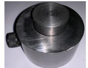
This is just a 1-inch rod sliding in a 1-inch hole. The set screw locks the rod at any height.
