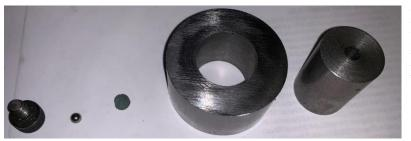
Here are all of the pieces. On the left is a scrap ¼-20 thumb screw. Next is an 1/8 inch diameter ball bearing. Then I have the puck of soft plastic.
