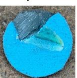
I cut a circle out and then used a razor blade to separate the resilient part from the fiber backing.
