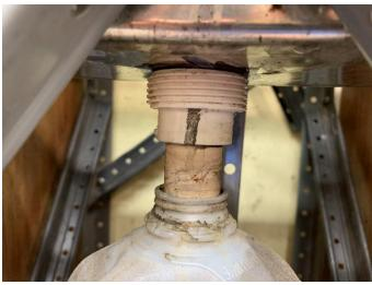
I selected a piece of ¾ inch schedule 40 PVC with half of a union welded on it³. This fitting has a circular groove with an O-ring in it.
