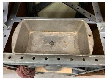
To convert the bread pan into a sink, I supported the ends on 2 by 4's. Then I took a steel cylinder about 1½ inches in diameter and placed it in the center of the pan. One whack with a large ball peen hammer and the pan had a nice slope to the center.
