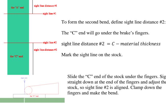
The "C" end will go under the brake's fingers. sight line distance #2 = C - material thickness(6)Mark the sight line on the stock.
