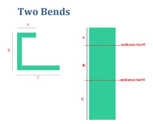
With two bends, there are three distances, A, B, and C, to the two mold point lines.
