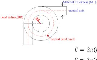
The bend allowance (BA) is  $\frac{1}{4}$  of the circumference of the neutral bend circle. If the neutral axis was at the centerline (i.e.,  $\frac{1}{2}$  of the material thickness), the circumference (C) would be:
