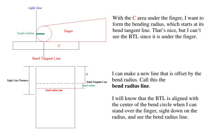
Given that section C is under the finger, the sight line distance (SLD) is:
