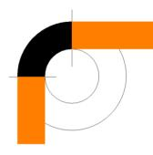
A practical bend includes a radius. If you tried to make a sharp 90° bend, the metal would likely crack.
