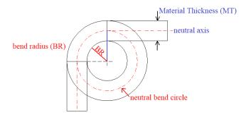
In the bend, the outside surface is stretched while the inside surface is compressed. Only along the neutral axis and the neutral bend circle is there no distortion.
