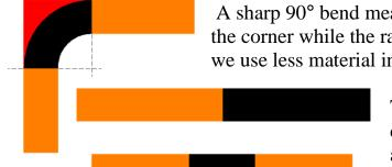
A sharp 90° bend means that the material must go all the way to the corner while the radius bend "cheats" the corner. Therefore, we use less material in the radiused bend than in the sharp corner.
