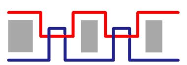
With the lock stitch, this force is concentrated at the point where the two threads lock together.
