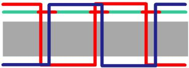
Then he sews right through the paper, which is represented by the gray rectangle. When done, the paper will separate at the line of holes and can be pulled out.
