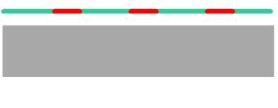
Nelson's second suggestion related to marking the path and location of the holes. He marks up a piece of paper and staples it to the material. The green line represents the line on the paper while the red dashes are the marks for the holes.
