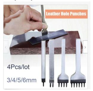
This one is for sale on eBay<sup>3</sup>. The idea is as simple as the Speedy Stitcher – place the material down on a board, align the fork along your line, and hit the end of the punch with a hammer. You instantly get up to 6 holes. Following up with the Stitcher should give perfect results.
