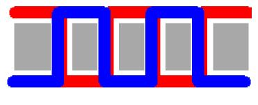
In Nelson's stitch, the thread bends at the holes in the material. As force is applied, the holes will elongate, and the bend of the thread will be gradual. This distributes the force, so the thread is less likely to break.
