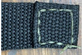
The back looks as straight as the front on three sides. The bottom line shifted. This must have been due to the needle not being perpendicular to the surface as I pushed it in.
