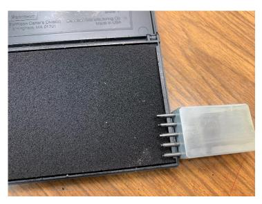
The plastic fork does work, but the tines easily bend. I made a replacement using a block of aluminum and some 4 penny finishing nails. The nails were first press-fit into the holes. Then I snipped them approximately to the same length. The belt sander finished the alignment.
