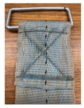
Time to try this technique on a folded back end with a captured ring.
