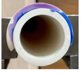
I then apply PVC cement. Since the patch encircles the pipe by more than 180°, it snaps in place.
