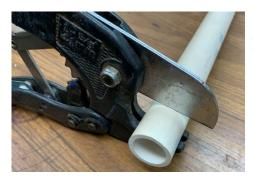
First, I snip off about 1-inch of pipe of the same diameter as being patched.
