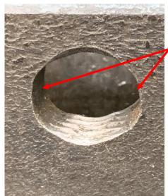
The hole in the movable jaw is first drilled and tapped to match the screw. A round file is used to remove the threads on the sides.
