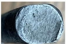
Looking at the end of the screw, you can see that the top and bottom threads have been removed.
