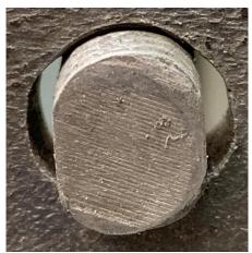
Rotate the screw  $90^{\circ}$  and the threads engage.
