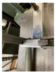
With the saw running, threaded rod is slowly fed into the blade. Care must be taken to prevent any rotation or the flat being cut will not be true.
