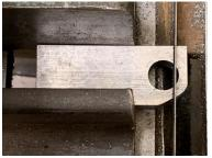
I started by going into my junk drawer to find a piece of stock with a hole that is a close fit to my threaded rod. Then, in the horizontal position, I sawed halfway through at the desired location.
