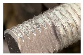
Sawing flats on threaded rod takes a bit of finesse. With plenty of metal on one side of the blade and almost none on the other, the blade will tend to wander off the part.
