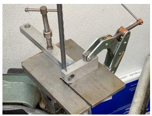
One clamp holds the block down while a second clamp, acting through a bar, prevents rotation.
