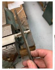
The stock was then clamped in my vise with the attached part sticking out. I used a file to bring the part to final size.
