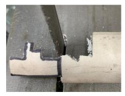
When I was done with all exposed edges and surface, I sawed the part free from the stock.
