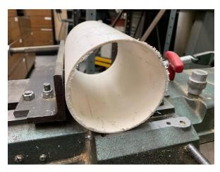
Sawing 4-inch diameter PVC sewer pipe on a horizontal bandsaw is trouble. It fits nicely in the vise jaws, but
