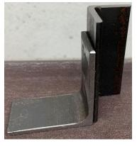
The basic idea is that the horizontal face is slowly abraded away by the belt as it remains in full contact. This sets the vertically mounted piece of angle stock perpendicular to the belt.
