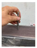
With my level of skill, trying to square up the end of a rod on a belt sander is hopeless. The belt is pulling the end horizontally while I'm trying to keep it vertical.
