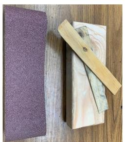
This tool also uses a 2 by 4 block. I calculated its length from the size of the 3-inch wide belt. Take the circumference and subtract 3-inches. Then divide by 2. For example, for a 21-inch belt, I first subtract 3 to get 18. Then I divide by 2 to get 9-inches.
