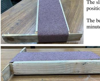
The slack reduced as I slid the second shim into position. The base of the shim faced the belt.
