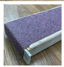
The fat end of the shim was cut such that about <sup>1</sup>/<sub>2</sub>-inch stuck out. This permits me to tighten the belt a bit more and also gives me something to grab when I need to remove the shim.
