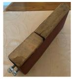
My first attempt at duplicating the sanding block involved two blocks of 2 by 4's and tensioning screws. The screws jack the blocks apart.
