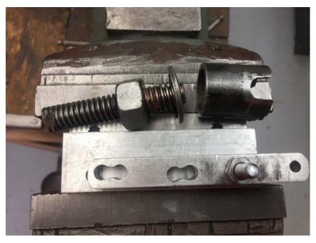
A short section of gas pipe proves the support for the jack. A length of Acme threaded rod and nut feed through a thick washer. The rod, nut, and washer are all well lubricated.
