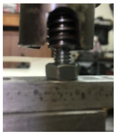
The threaded rod passes through the washer and the pipe. Here I have screwed the threaded rod into the top of my stud. The ½-20 nut is finger tight.
