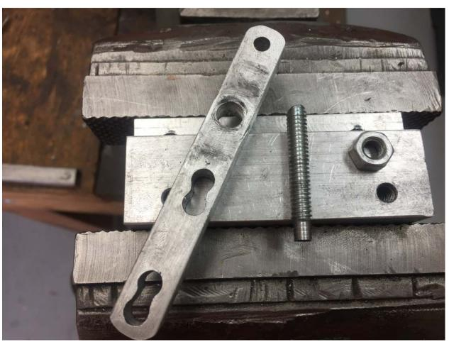
I have a block with a threaded hole in it, a length of threaded rod, a bar to be bolted to the block, and a nut.
