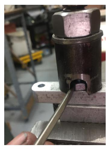
With the stud tensioned, I used a small screwdriver to nudge the nut snug against the bar. Then I loosened the big nut and removed the tool.
