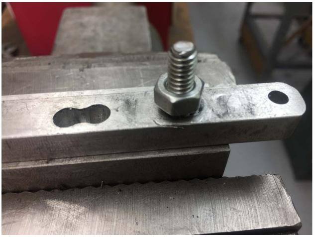
I thread the stud into the block, drop on the bar, and spin on the nut.
