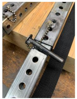
Securing each leg is a 3/8 inch diameter pin with a washer welded on top. Epoxied under the washer is a neodymium magnet that reduces the chance of the pin falling out. The ball chain is braised on. Place the pin through a hole in the larger tube and the legs are adjusted in steps of 1 inch. Place the pin through a hole in the smaller tube and the 1 inch steps are offset about  $\frac{1}{2}$  inch. In this way, each leg can be independent adjusted to the nearest  $\frac{1}{2}$  inch.
