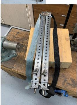
The bipod is built of square tubing designed to nest.
