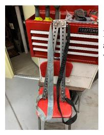
By adjusting the overall length of each leg, I am able to adjust the amount of slack in the straps. Here you see the legs fully collapsed which give the most slack.
