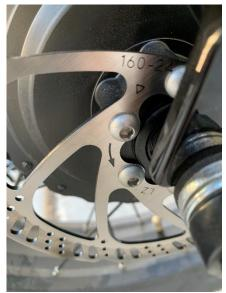
The disc brakes on my bicycle work best when the gap between brake pads and rotor is near zero. If the rotor is dead flat, the pads can be set barely above the surface. This would provide the least travel on the brake lever before braking starts. It also gives most of the brake lever range to driving the pads into the rotor.
