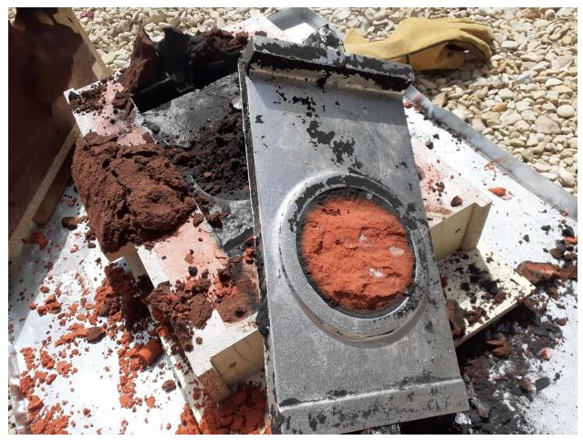
I used oil based molding sand. Here you see one of the two side plates. The hole has a raised lip which is an improvement over the plans from Mr. Gingery.
