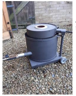
Casting parts for my shaper demands a furnace. Mine burns waste oil.
