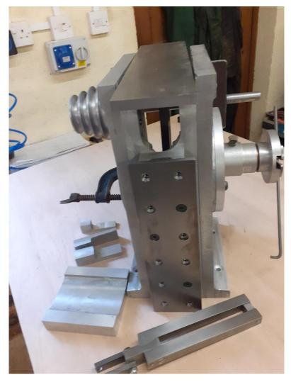
While all aluminum parts were cast, the steel parts were machined from bar stock.
