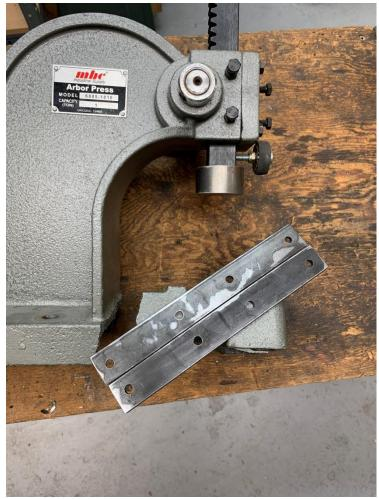
Why not try bolting on side straps? I made two from 1/8" X 1" X 8" CRS. The casting will prevent the strap from twisting, and the one inch of steel is extremely strong in sheer. I selected 5/16 bolts to have about the same strength in sheer.
