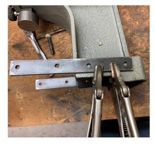
I aligned the first strap, by eye, on the rear part of the casting. Then I match-drilled the two holes using the F drill.
