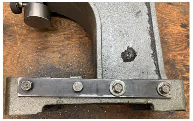
With the two casting parts pushed together, I clamped the first strap. Then I repeated the match-drill and tap process.
