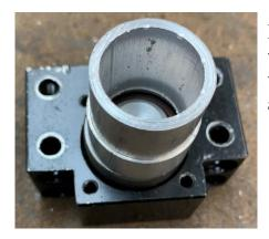
I pressed out a bearing from this block yesterday, and it went well. The trick is first to heat the aluminum block with a hot air gun. My 1-ton arbor press pushed it out with a gentle push on my 2-foot-long cheater bar.
