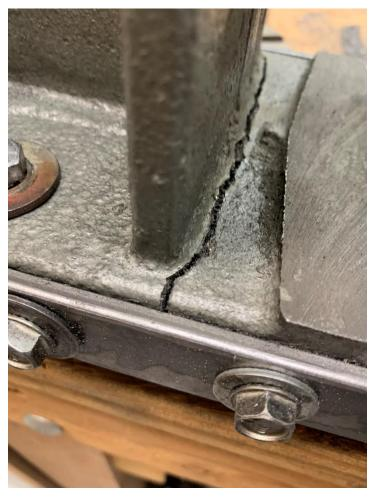
I torqued down on all bolts and then applied about as much pressure to my cheater bar as caused the failure.
