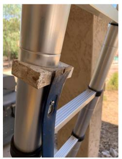
and gently pulled the dent out. I took special care to spread the force from the end of the prybar over a large area so as to not create a new dent.
