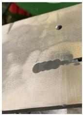
After degreasing the slot, I put a piece of painter's tape on the backside. This was backed-up with a magnet. Then I pushed JB Weld into the slot and struck it off.
