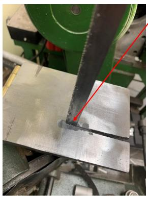
With the table all the way down, the blade slot is precisely in the right place. Notice how far off I was with my series of drilled holes.
