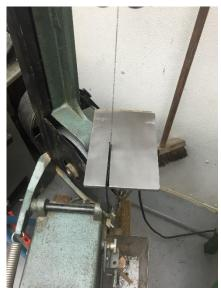
This flip-up table<sup>2</sup> on my horizontal/vertical bandsaw has served me well. Then I decided I wanted the blade to align with the edge of the table. That was when I started to make a mess. Not only was I not able to get that alignment, but I also enlarged the slot around the blade to the point where small pieces of sheet metal were getting sucked down into the lower blade guide.
