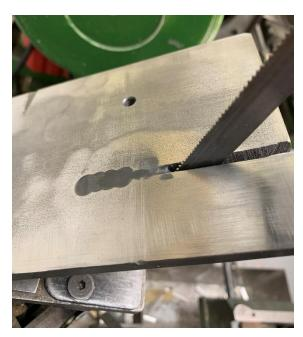
My solution was a bit unorthodox. First, I unplugged the saw. Then I turned the blade around, so the teeth were facing towards the back of the saw.
