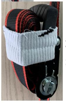
Slip the band of cut up sock around the strap and the handle of the ratchet.
