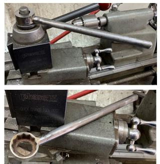
I didn't have the correct size box wrench to modify but did have a spare socket. Since the torque requirements were modest, I silver brazed a steel rod to the outside of the socket.
