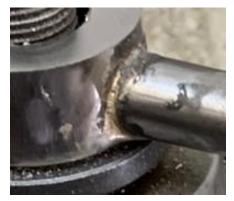
First, I cut a radius into the end of the rod to slightly less than the OD of the socket. The braze filled the void to provide a strong joint.
