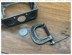
It doesn't matter if the anvil of the clamp is larger than the punchout since you are pushing into the box. Just be sure the foot is smaller.
