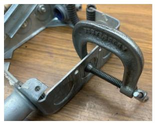
An easy way to get leverage on the punchout is to use a C-clamp<sup>2</sup>
