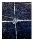
Push down on the punch, and you have a divot right at the intersection. The point of a small drill will drop into this divot. For larger drills, the divot can be enlarged with a bigger spring-loaded punch.
