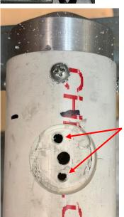
My solution is to first drill two holes roughly on a diameter while drilling my pilot hole.
