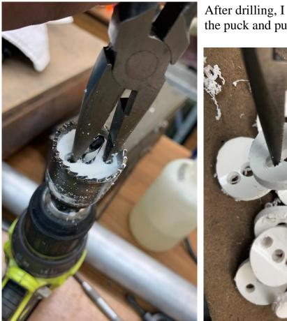
After drilling, I use a needlenose pliers to grab the puck and pull it straight out.
