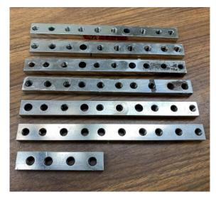
About 25 years ago, I found about a dozen of these chrome plated steel bars in the trash. Each one was drilled and tapped  $\frac{1}{4}$ -20. They are  $\frac{1}{4}$  inch thick,  $\frac{1}{2}$  inch wide, and 6 inches long.
