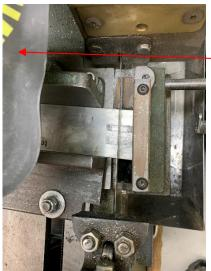
With the movable jaw pushing on the edge of the stock, I lowered the blade in preparation for cutting. I'm using my AirShim<sup>5</sup> to slow the downward feedrate. This is necessary in order to minimize both the burr on the bottom edge plus error due to excessive feed rate.
