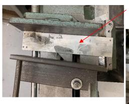
I placed a piece of scrap 1/8 inch thick, 2 inches wide stock against the fixed jaw.
