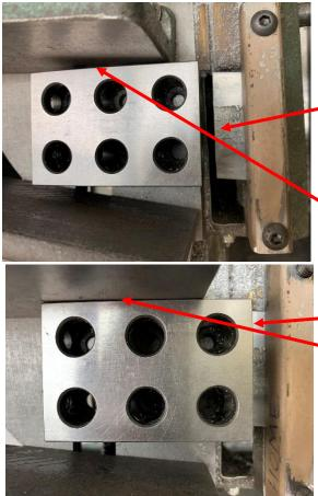
Even though the stock was way out of alignment, the saw cut will be aligned with the blade to within the repeatability of the saw and straightness of the cut.
