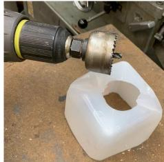
Using the larger hole saw, drill through the top. I found a web bridging a V gap in the bottom. Snipping that web out made it easier to start the drill near center.
