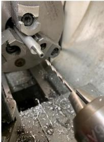
Next I spot drilled the end followed by drilling in about 1-¼ inches with a 1/8 inch drill. Fed in about 1/8 inch at a time, retracted, and cleaned out the swarf embedded in the flutes of the drill. Used cutting fluid.
