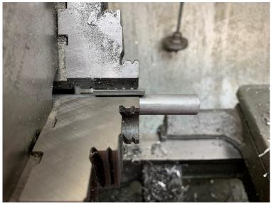
The stock is placed in my 3 jaw chuck with a 0.1" spacer between one jaw and the rod. This packing offsets the rod. The stickout is around <sup>3</sup>/<sub>4</sub> inch.
