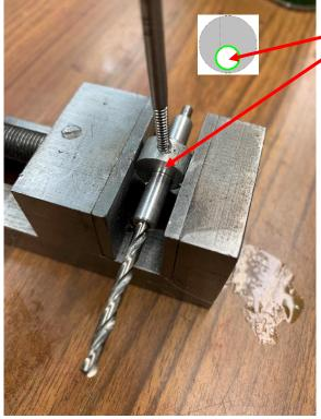
Moving over to my Drillpress, I first aligned the part in my vise so the spigots were at the bottom. This gives me the maximum amount of metal above the axial hole for tapping. I used a #36 drill to cut a hole down to the axial hole.
