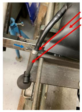
Here is the bleed valve installed between the Air Shim and new length of tubing. Gently tightening the screw (blue arrow) all the way down restores the Air Shim to normal operation. Backing it out just a little gave me the right amount of air bleed to lower my bandsaw blade at the desired rate.
