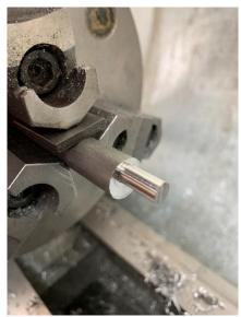
Most of the turning was interrupted cuts which slam into the cutter on every revolution. To reduce this jolt, I fed in only 0.01 inches per pass until most of the surface was being cut. Then I fed in 0.025 inches per pass. Machining stopped when the diameter of the spigot was about 0.01 inches larger than the inside diameter of the tubing I had chosen. Overall length was about <sup>1</sup>/<sub>2</sub> inch.
