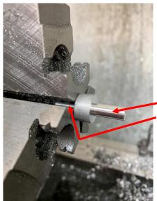
I needed to machine the second spigot so it aligned with the first spigot. Not a problem. Just held the part by the first spigot and took light cuts. If the 1/8 inch drill had not gone through this end, I would have spot drilled and drilled deep enough to get a through hole.
