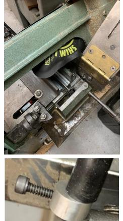
By using an "AirShim" which I bought at Home Depot for \$15 plus a small modification, I can limit the feedrate on my horizontal bandsaw. To see it in action, go to
