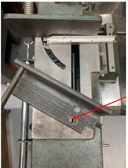
My movable jaw is free to pivot a lot more than necessary. As I crank it in, I have to periodically stop and move the left end closer to the fixed jaw.
