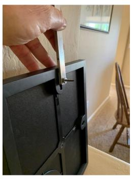
To use the tool, slip the blunt end of the threaded rod into the top end of the keyhole slot.
