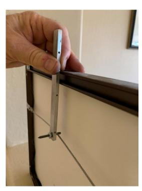
If the picture is supported by a wire, hook the blunt end of the threaded rod under the center of the wire, lift up, flip the picture over, and again use the bar to snuggly push the point into the wall. Lift the picture away and push the point in deep enough to leave a mark.
