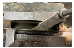
The table was drilled and tapped to accept the bolt. This hole can also be used as an anchor point for an outboard hold down clamp.
