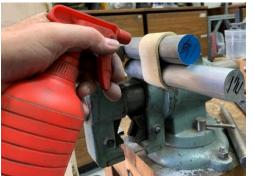
Spraying the plastic with water quickly hardens it. I repeated the process with the other piece of PVC.
