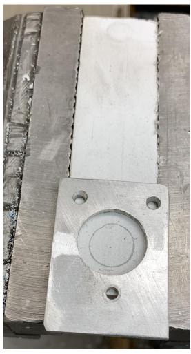
My next tool was formed from a piece of scrap 1/8-inch thick aluminum plate - I drilled a 7/8-inch hole in it. The pipe is a loose fit.
