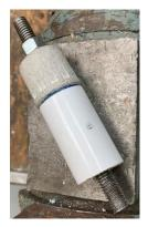
I built this tool that permits me to spin the PVC pipe. It consists of a ½-inch schedule 40 end cap and coupler.
