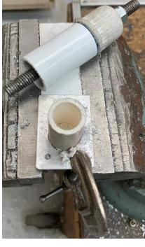
I only needed to run the drill for a few seconds while pushing down to accomplish the weld. I go in about 3/4<sup>th</sup> of the way through the board.
