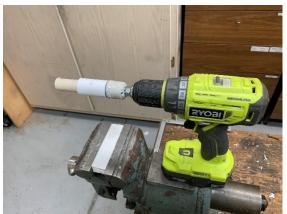
Here I have loaded in a short piece of PVC pipe.
