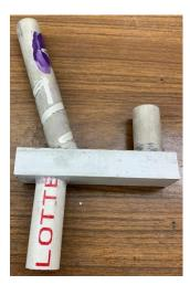
It is possible to directly weld PVC pipe to PVC trim board without first drilling a close-fitting hole. And you don't need to use PVC cement.
