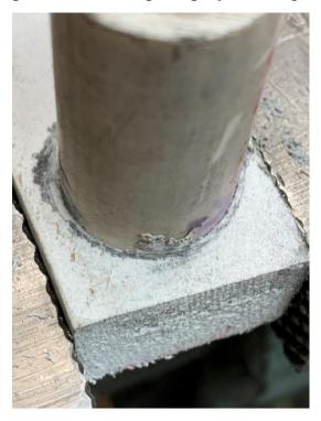
This close up shows bits of swarf that were caught between the pipe and the plate. They can be removed with a sharp knife.
