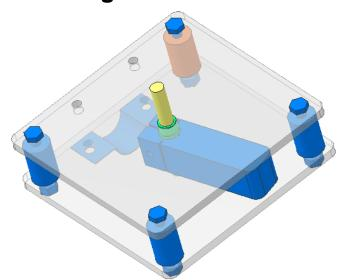
In this overview rendering I have made the two aluminum plates translucent. You can see the spinning bar, the handle clamp, plus one of the bronze bearings (green).
