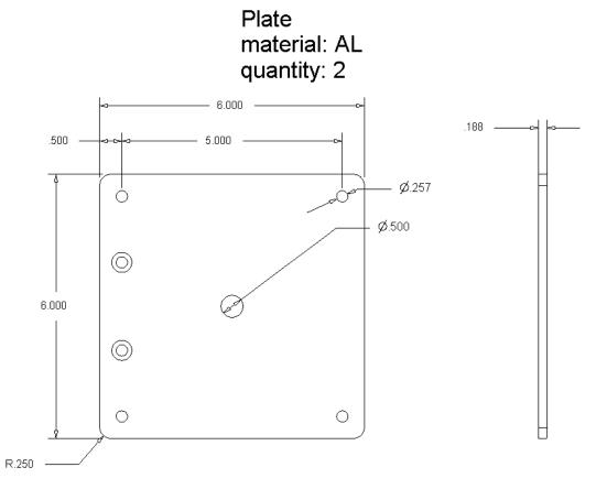
Hint: cut the plates, clamp them together, and then drill all holes. Before unclamping, mark the position of one plate relative to the other so they can go back together the same way. All holes will then perfectly match.
