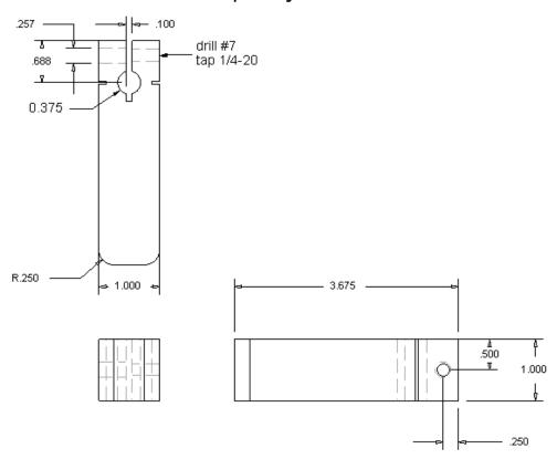
A ¼-20 bolt threads through to clamp the shaft. I put a nylon lined lock nut on the outside. The three relief cuts are needed to weaken the bar enough to clamp the shaft.
