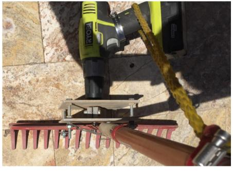
You can see the bar which is clamped onto the shaft. The front two bolts pass between rake tines and are secured with washers. The back two bolts anchor bailing wire which prevents the plates from lifting up. That nylon rope prevents the drill from spinning. The hose clamp around the drill handle depresses the trigger.
