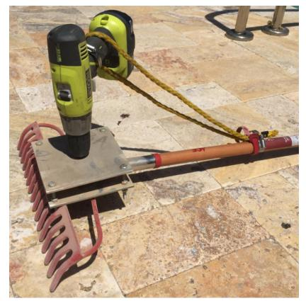
The two 3/16" thick aluminum plates support a spinning bar plus protect the user. In the first complete design there will be sheet metal around the perimeter to full enclose the bar.
