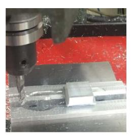
I CNC machined 41 dimensions of varying sizes. Thirty five of them were with the cutter diameter defined as 0.250 inches. This generated a constant offset in the data. I then changed the cutter diameter in the g-code to 0.248 inches and took 6 more data points.
