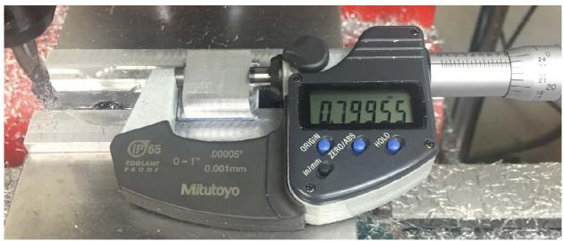
I used a digital micrometer able to read down to the nearest 50 millionths of an inch.
