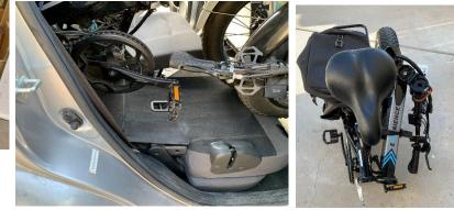
when it is folded, the cranks become a problem. They freely turn in the reverse direction but jam in forward when the back wheel can't turn. The cranks can also jam into part of the frame or handlebars when the bike is folded, preventing the bike from rolling forward.
