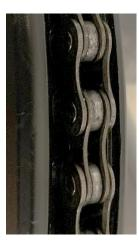
The chain is now in the gap between the sprocket and the chain guard. With the back wheel fixed, you can freely turn the crank in either direction.
