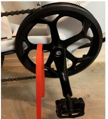
This is a potentially dangerous condition. If you jump on the bike and push down hard on a pedal, it will offer little resistance and could throw you. I remind myself that I'm in neutral by looping the tool through the sprocket spokes.
