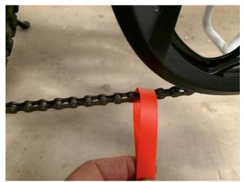
To take the bike out of neutral, wrap the tool around the chain and pull horizontally about <sup>1</sup>/<sub>4</sub> inch. The chain should shift back onto the front sprocket as you start to turn the crank counterclockwise. Listen for a clatter as the chain engages with the sprocket.
