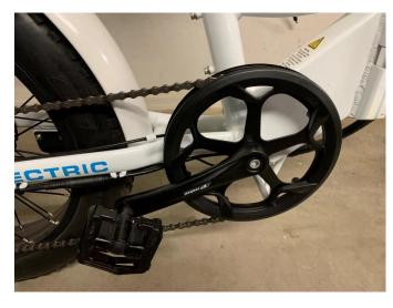
The front sprocket has a chain guard around it. The chain engages with the sprocket while being flanked by the guard.
