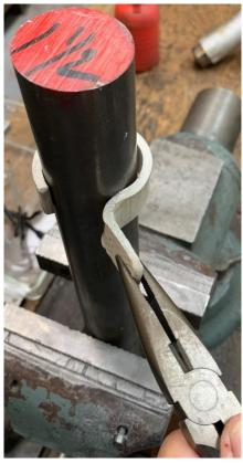
Using a piece of 1½ inch diameter round stock as my mandrel, I heated up the plastic while holding it with plyers.
