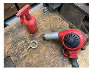
The trick is to heat the plastic up with a hot air gun until it is pliable like thick leather. Then it can be molded by hand. I use my bare hands, but if you are sensitive to heat, gloves are enough to protect you.
