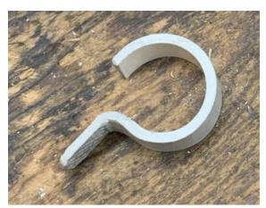
This is an early model. Notice that the inside diameter is distorted. I just need to remold it.
