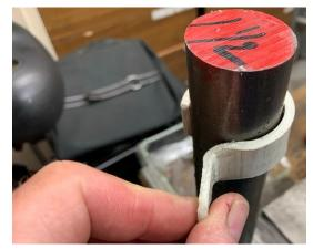
Once the plastic became soft, I squeezed it onto the mandrel and then sprayed on the water.
