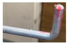
I coat the end of the "L" shaped rod with the release agent and also hold it in my pin vise.
