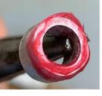
The first step is to evenly coat the lower mold with the release agent. This is accomplished by coating the end of the ring. There must be no bare spots but I don't need to worry about having too much.
