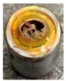
I again preheat the mold with my gun, apply hot glue into the mold, and formed a cone. After it cooled, I pulled the mold off of the rod. The bit of flash over the hole is harmless.
