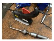
Of course, I need my hot glue gun. I also need a length of <sup>1</sup>/<sub>4</sub> inch diameter rod bent in an "L". I'm holding it in my homemade pin vise because it will get rather warm.
