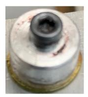
After applying heat, you can see the excess glue forms a ring around the mold.
