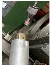
Then I use my heat gun to warm the lower mold. If in doubt about how much heat to apply, put a dab of hot glue on the mold. When it melts, it is ready.
