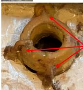
To form extension arms, use a saw to cut radialslots through the mold's wall.
