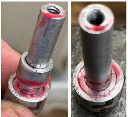
After pushing the ring down into the lower mold, I rotate it a bit. This evenly distributes the release agent into the mold plus forces it against the inside bore and the bottom.
