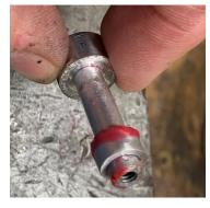
The ring slides onto the shaft with the greased end facing the lower mold.
