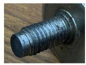
Then I spun on a nut as a guide and filed off the last ¼ inch of thread. This made it easier to align the new nut by feel plus require fewer turns to snug it up.
