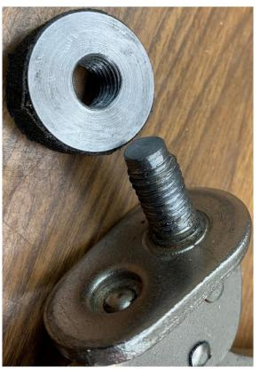
My new nut was made from a scrap of 1-1/4 inch diameter mild steel from my junk drawer. The hole was drilled 27/64 and then tapped 3/8-16. I spread Go2 Glue on the OD and attached a strip of emery cloth. You can see that it bunched up a little but I was able to cut out the bulge and add more glue.
