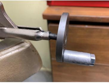
The adjustment screw was fitted with a disk of mild steel I found in my junk drawer.
