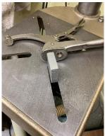
You then place the clamp at 90° to the slot in the Drillpress table and
