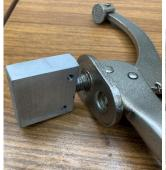
Björn suggested replacing the spin-on nut with a fixed bar<sup>4</sup>.
