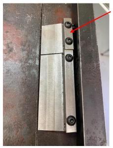
I installed another bar to a plate that was half as wide. The button head screws are again  $\frac{1}{2}$ -inch from the ends, and the 10-32 set screws are  $\frac{1}{4}$ -inch from the ends.
