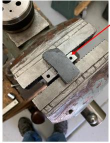
I stuck the magnet to the bar and placed it between the vise jaws. This ensures that the top of the bar is flush with the top of the vise jaw. After tightening, I removed the magnet.
