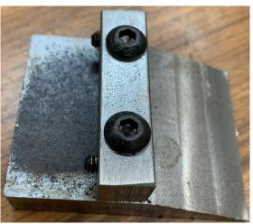
I tapped the second hole and deburred it. Then I ran the second button head screw, sawed off the end, and sanded it flat. And finally, I ran two set screws in those horizontal holes.
