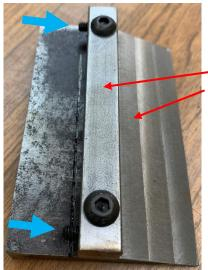
The part I am fabricating is unimportant. I want to focus on the steps I used to drill and tap the holes that secure the bar to
