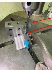
Going back to my drill press, I used a 1-2-3 block to align the end of the bar with the flank of the plate while having the #4 drill down the hole. I eyeballed the edge of the bar, so it is aligned with the transition from sloped to flat (blue arrow).
