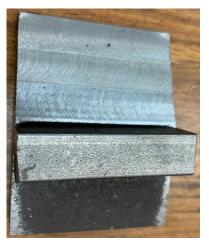
I cut the <sup>1</sup>/<sub>2</sub>-inch by <sup>1</sup>/<sub>2</sub>-inch bar on my bandsaw using the plate as my length gage. You will see that a recurring theme is that I try to avoid measuring.
