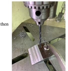
After clamping the plate down, I removed the bar, used my spotting drill, and my #4 to go through the plate.
