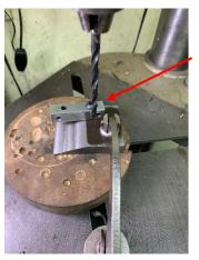
Next, I loosened the screw, swung the bar away, and tightened the screw. I do not want that bar swinging into the drill bit as I cut my second hole in the plate.
