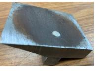
After sawing the excess screw off on my bandsaw, I sanded it flat on my belt sander.
