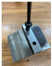
I'm running a <sup>1</sup>/<sub>4</sub>-20 button head screw down the tapped hole until it is tight.
