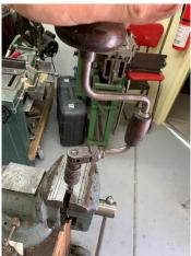
After tapping the hole, I used my brace-and-bit fitted with a countersink to deburr.
