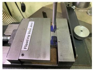
After clamping in my bar, I installed a spud<sup>4</sup> and located its point into the punch mark. Then the fence was set against the vise and locked in place.
