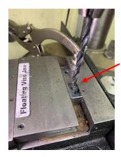
I then slide the vise along the fence with the spud installed and stopped at my scribed line.
