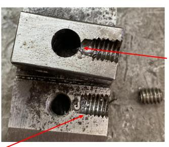
I removed the button head screw to inspect the blind tapped hole. You can see that I was able to drill down to the <sup>1</sup>/<sub>4</sub>-20 screw but did not damage it.
