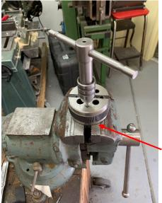
After coating the tap with cutting oil, I passed it through the bench block and into the bar. This keeps the tap vertical as I cut the threads.
