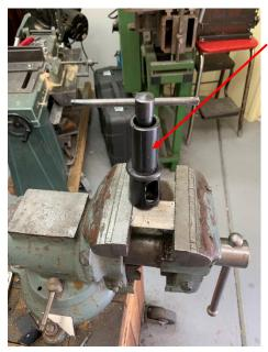
My ¼-20 tap was fitted into this tap handle with built-in base. After aligning the top of the plate with the top of the vise jaws using my magnet trick, I tapped this first hole. Then I deburred it with my brace-and-bit.
