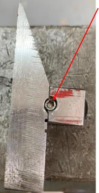
I screwed in a 10-32 setscrew that was <sup>1</sup>/<sub>4</sub>-inch long. This acts as a key to prevent the block from rotating relative to the plate.
