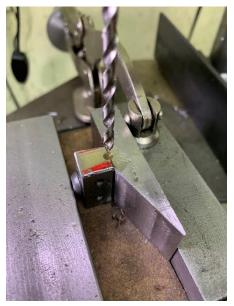
I fitted the block on the plate and placed it in my drill press vise on its side. Then I used my spotting drill to cut a cone at the joint between the block and the plate.
