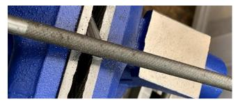
Using a fine file ¼ inch in diameter, I cleaned up the cut.
