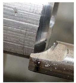
That got me thinking about making my own corner radius tool. The radius here is about <sup>1</sup>/<sub>4</sub> inch. The cutter is made from water hardened rod but since I'm cutting aluminum, I didn't harden it.
