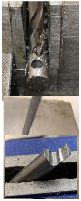
Next, I cross drilled with a sharp 1/8 inch drill. Used plenty of CoolTool.
