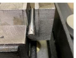
After sawing off a 2-inch piece of rod, I clamped it into my small vise which was then clamped into my drill press vise. I chucked up a piece of ¼ inch diameter rod and lowered it into the gap between the vise jaws. This gave me my center. Using plenty of CoolTool, I drilled this divot with my spotting drill.
