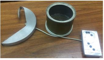
The first step is to wrap the cable around a round object with a diameter about half of the desired diameter. Weight the ends of the cable and make snug.
