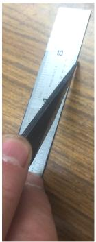
The flat face goes against my straight edge. This protects the straight edge from nicks. The beveled edge tends to apply a small force that keeps the knife against the straight edge.
