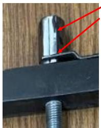
My version of this end was cut from ½ inch hex CRS. I cut the groove and drilled and tapped a center hole to a depth of ½ inch. Then I silver soldered the end to a 15-inch long ¼-28 ready-rod. Locktite Red would have probably held, but soldering is quicker and stronger.
