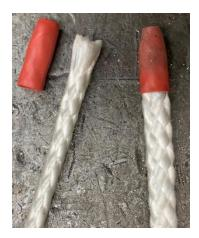
Here are two test samples. I used a heat gun on the left sample. When cool, the heat shrink pulled right off, revealing un-melted line underneath.
