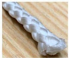
Cut the end of a plastic, woven line, and you are greeted with a little cloud of fibers.
