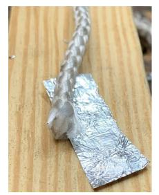
I start with a piece of aluminum foil. The width is about three times the diameter of the line. The length should be enough to wrap around the line a few times.
