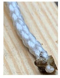
A common remedy to the little cloud is to roast the end over a flame. This melts the plastic and forms little blobs. The line is sealed, but you may have some sharp ends to contend with. They can hang up on the line while tying knots.
