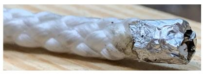
You are left with a rigid, uniform cylinder coated with aluminum foil: no sharp edges and no loose ends.
