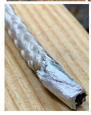
Peel as much of the aluminum foil off of the line as possible. Expect to find foil that is solidly fused to the line.
