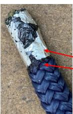
After it cooled, I peeled off as much of the foil as possible. The end of the line fully melted. However, this does look ugly.
