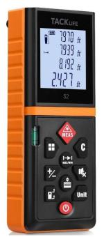
Recently I took a chance on a \$30 laser measuring tool<sup>2</sup> which claimed to be accurate to  $\pm 1/16$  of an inch (1.5 mm): the TackLife S2 Laser Distance Meter<sup>3</sup>. The display has a minimum increment equal to this claim of accuracy. It can measure distance, area, perimeter, volume, and, indirectly, height. Below 2 inches, I get an error message. The claimed maximum distance is 130 feet but I have no way to test that.
