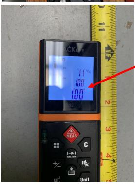
I then switched to my steel ruler on the floor of my shop. Due to variations in the floor, I had to prop up the end of the meter to keep the laser pointer at the correct spot on my target.
