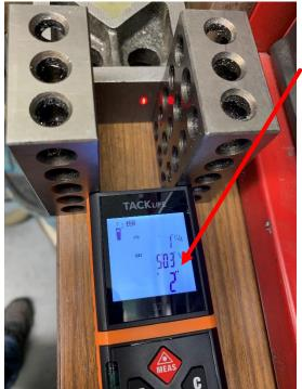
Using my 1-2-3 blocks, I set the distance from the front face of the meter to the base of a V block.
