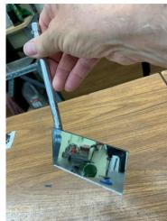
I glued<sup>2</sup> a ½-inch ball bearing to the back of a mirror near the corner. Then I glued a countersunk neodymium magnet to a scrap of angle that was first brazed to a rod.
