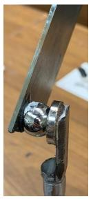
The countersink in the magnet makes a nest for the ball. As long as both the ball and magnet are free of oil, it holds well. I can angle the mirror as needed relative to the rod.
