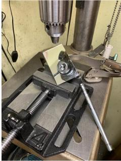
The inspection mirror, steadied by the magnet attracted to the vise, makes it easy to see the jaws while inserting the drill bit.
