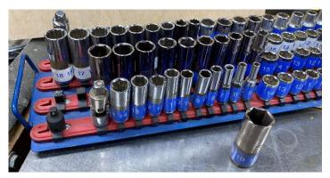
For the way I work, I like taking an entire set of a tool type to the work. I hang the socket board on the outside of my toolbox to increase direct access and to conserve space in the drawers. On the board, there are separate socket rows for 1/4", 3/8", and 1/2" drive. The large labels on each socket are MUCH easier to
