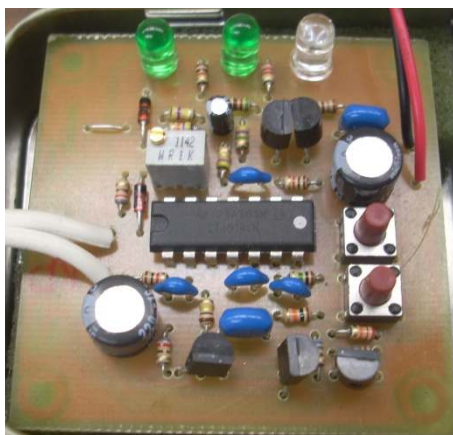
This is the first hand etched and drilled prototype that used almost the same artwork except is single sided. I didn't have an amber LED so used a green one for the center LED.
