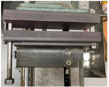
To use, I drop in the fixed jaw. The plate on the right end aligns with the slot under the blade. I then slide in the movable jaw until it touches the bar on the left end of the fixed jaw.
