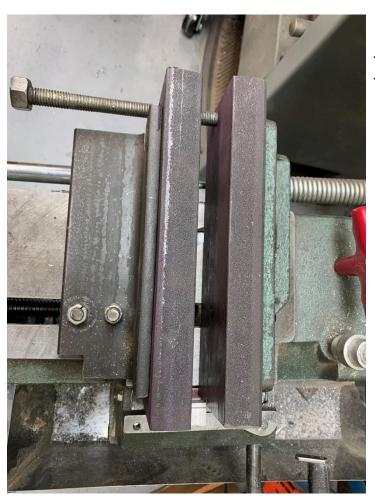
The third feature is a quick-adjust jackscrew. I have one on my regular jaws, and it is useful. I tap drilled ½-13 through the end of the bar such that the threaded rod is also a stop for the movable jaw. Then I clearance drilled ¾ of the way through. Tapping ½-13 in steel is hard work, so I didn't want to cut any more threads than necessary.
