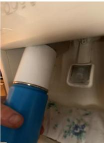
The coupler is a loose fit to the outside of the water bottle's mouth and the chute. The length of the coupler is enough to hold a bunch of ice cubes when they jam. I can then lift the coupler away from the chute, and none escape. A little jostling and they all go in my bottle.
